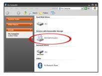
4. Run the "setup.exe" file located in "PCIe USB 3.0 2Port Card (PEXUSB3S2)". Follow the on screen instructions to complete the driver installation.
